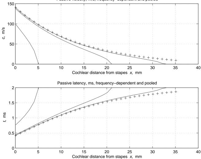
Passive velocity, m/s, frequency-dependent and pooled
